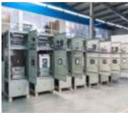
Automatica medium voltage cells for 24kV electrical stations. Transelectrica - Romania.
